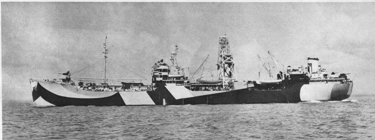
Supplying pure water to invasion troops is an important function of this auxiliary ship, an AW. Tall jimmy-legs crane between stack and
